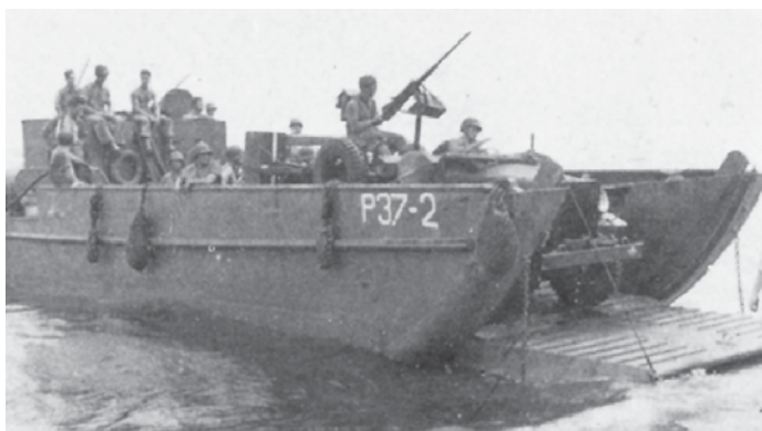
13. Američki desantni brod LCM-Mk2 sličan onima pronađenima na morskom dnu (izvor: http://www.ibiblio.org/hyperwar/USN/ships/ships-lcm2.html ) / US Landing craft LCM-Mk2 similar to the ones discovered on sea bottom (source: http://www.ibiblio.org/hyperwar/USN/ships/ships-lcm2.html )
