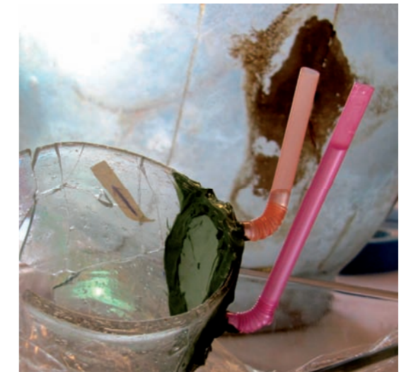
Figure 12. Integration using epoxy resin with the aid of a silicone mould (Photo: M. Ćurković)
