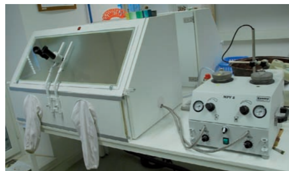
Figure 9. A micro sandblasting device and chamber (Photo: A. Jozić)
