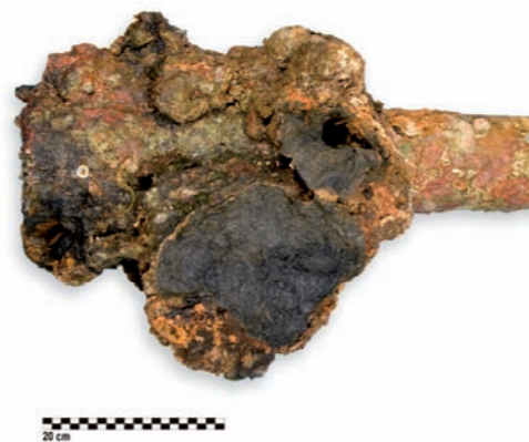
Figure 3. Black sediment created by the decay and decomposition of iron (Photo: M. Mustaček)
