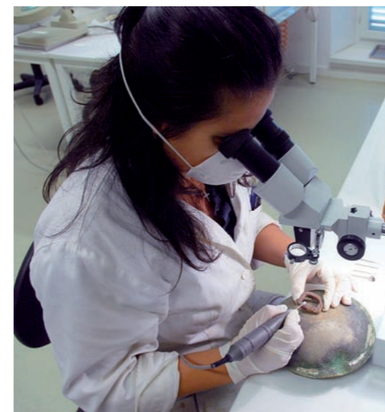
Figure 10. Mechanical cleaning an iron object under a microscope (Photo: M. Mustaček)
