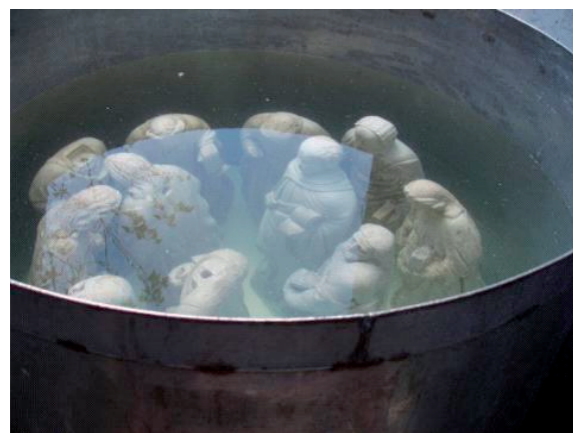
Figure 2. An example of desalination by submersion in a vat (Photo: I. Martinović)
