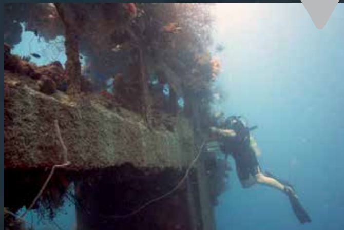
► 8. Shinkoku Maru showing loss of hull plating after 75 years of corrosion / Gubitak oplata trupa olupine Shinkoku Maru nakon 75 godina korodiranja (Photo: A. Selman)
