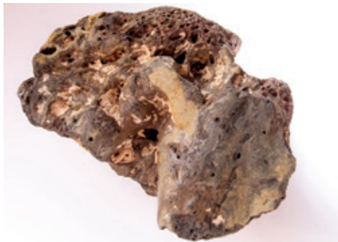
Figure 31. Molten brick with traces of glazing (photo: L. Bekić)
